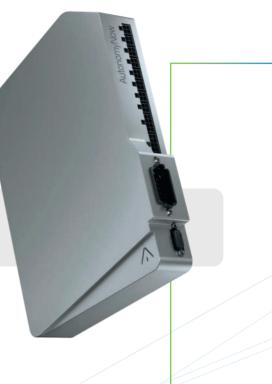
Advanced radar is designed for commercial vehicles and boasts a wide angle of 100 degrees, which allows it to follow up to 250 objects within a 170 m radius. The radar measures the range, radial velocity, linear and horizontal angles, reflectance and other parameters of objects, which can occupy up to 10 traffic lanes.
