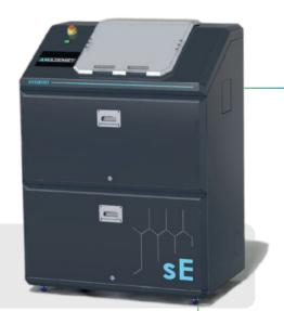
SafeEtch technology is innovative because it automatizes the processing of metal 3D prints - such as the removal of support structures, surface treatment, and removal of loose adhesive pow-ders.
