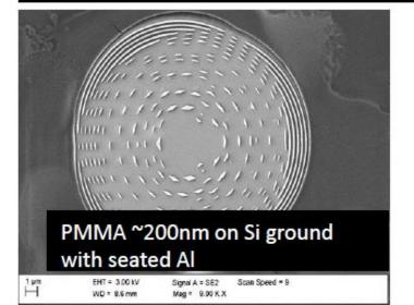
PMMA on Si substrate with Al. Fourierowski phase hologram – gray
